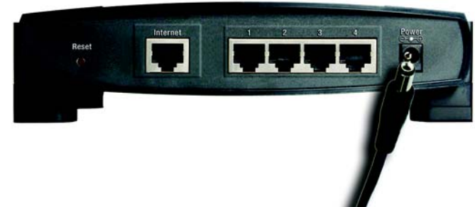
Figure 4-4: Connect the Power
